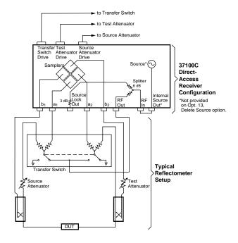
A Reflectometer test set is available as a special option for the 37100C. It contains the transfer switch, both attenuators and couplers. It also offers two bias tees and a front panel amplifier loop for active device testing. As compared to a 37300C VNA, the output power and hence the dynamic range are degraded by 10 dB typically.
